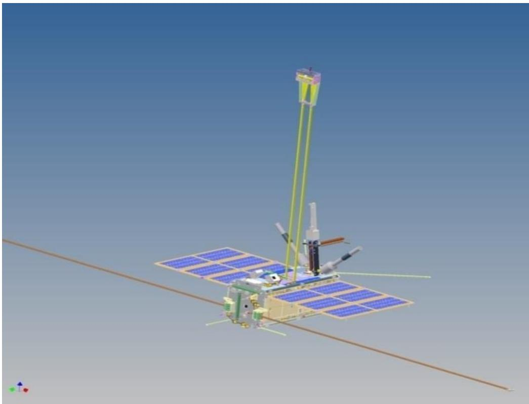
**Figure 4.** General view of «Chibis-M» with open antennas and solar panels
