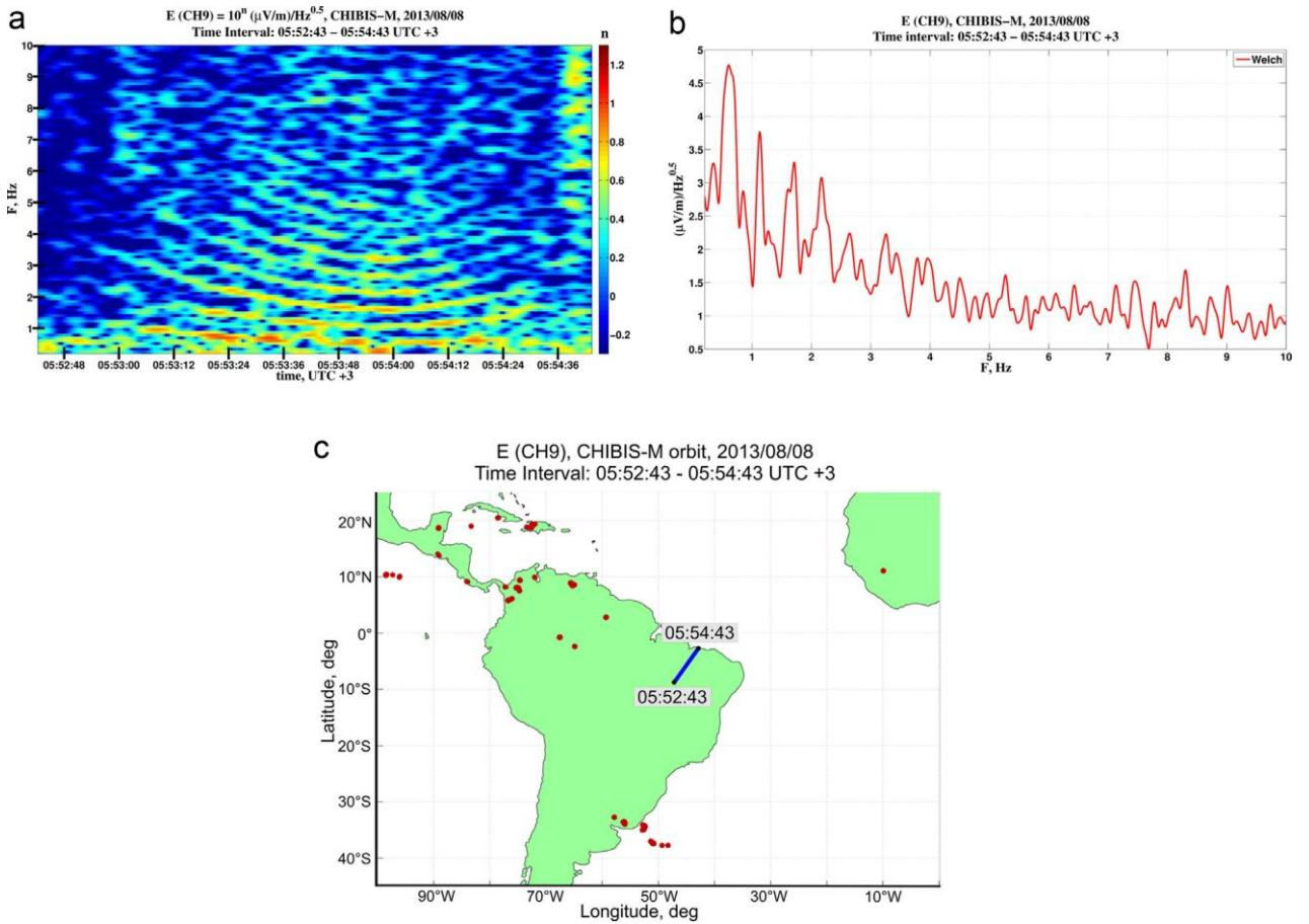
**Figure 8.** (a) Dynamic spectrum of electric component of “fingerprint” emission detected on 2013/08/08 starting 05:52:43MST. (b) The Welch spectrum of electric field variations recorded on 2013/08/08 (shown in (a)). (c) The vertical projection of the Chibis-M orbit during ULF emission observation, superposed with lightning activity, as identified by WWLLNarray.
